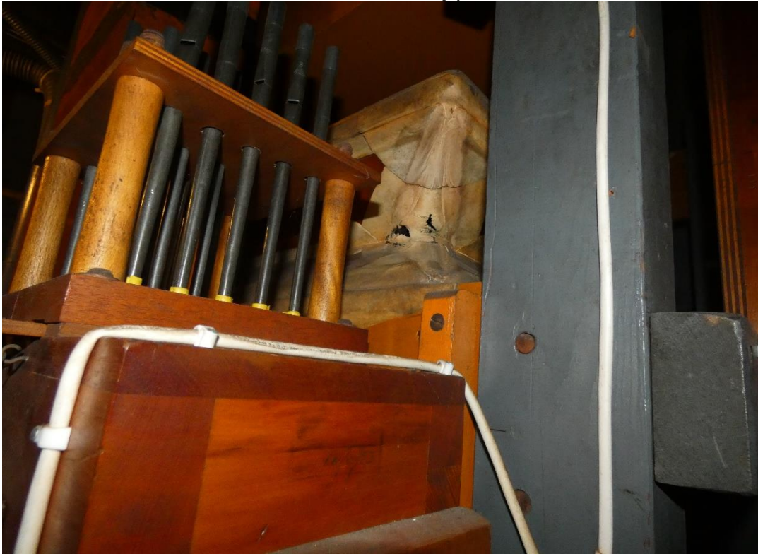
Perforated corners on the Reed heavy pressure reservoir.
