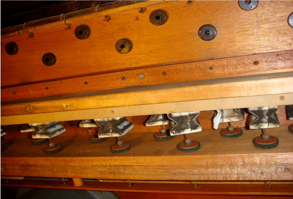
View of the Swell key action showing chest magnet primary and secondary motors.
